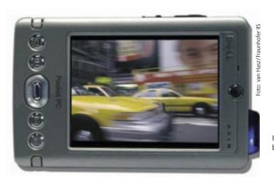
High-quality movie playback on mobile devices sound at very low bit rates. Thus, a total bit rate of only 500 kbit/s is sufficient for ISMA 2.0 compliant streaming of video in TV size and surround sound.
