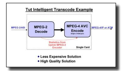
In some digital headends, more than 70% of the channels in the service provider's channel line up is pre-encoded, digital content coming from satellite feeds. These channels are pre-compressed using MPEG-2 to facilitate efficient transmission over today's satellite networks.
